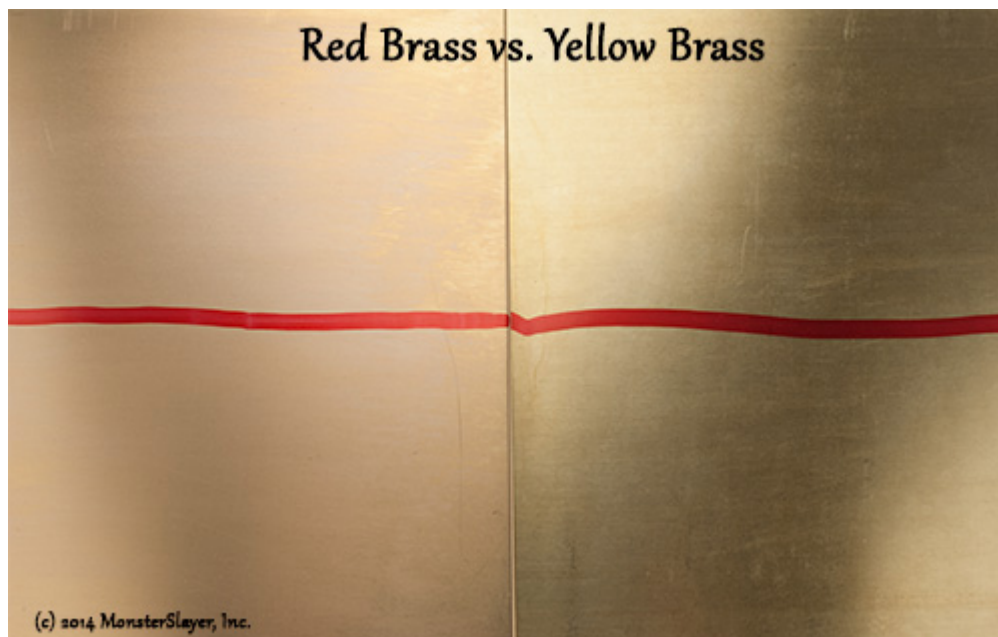
Figure 3. Color difference of copper-zinc alloys (www.Monsterslayer.com 2015)
