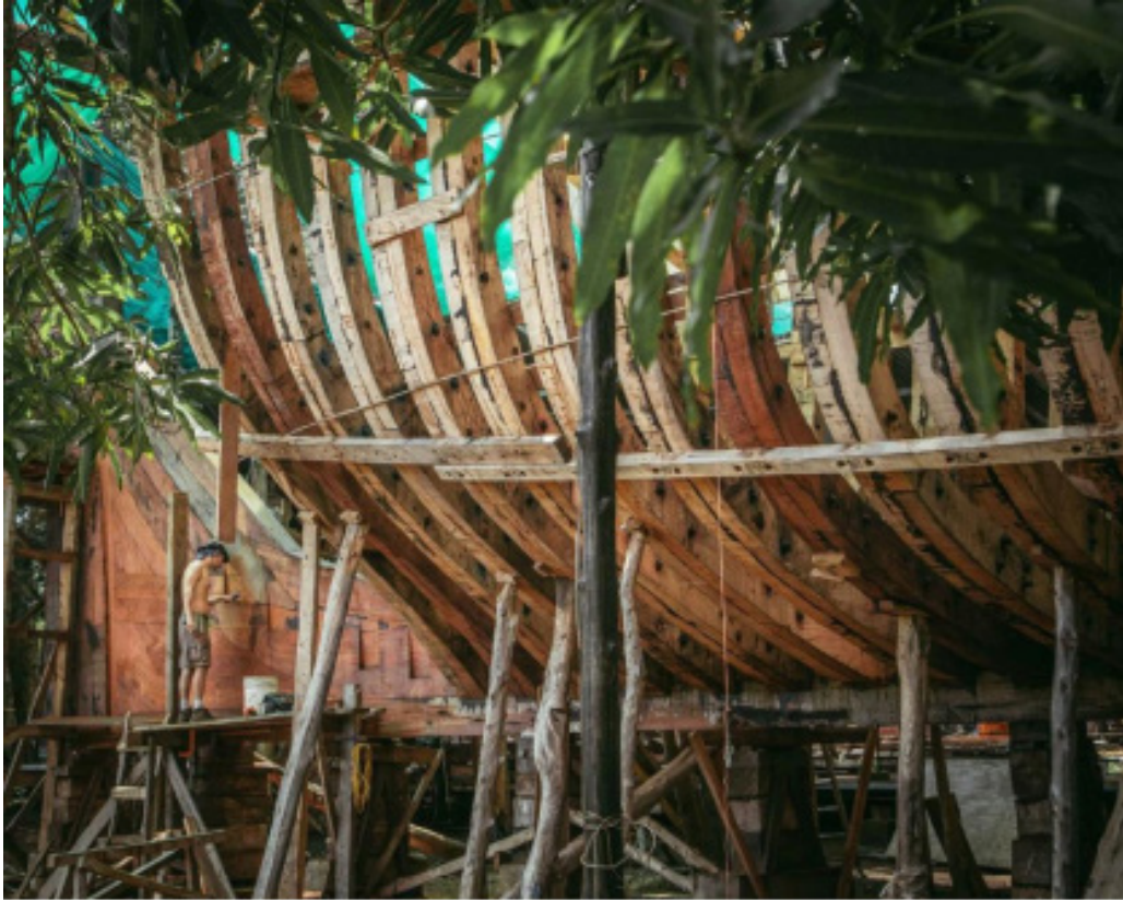
Figure 14. The huge all-timber ship, Ceiba , being completed in Costa Rica, uses a local variety of tamarind timber ( Tamarindo del Monte ) in its construction. Image courtesy of the Sail Cargo project.
